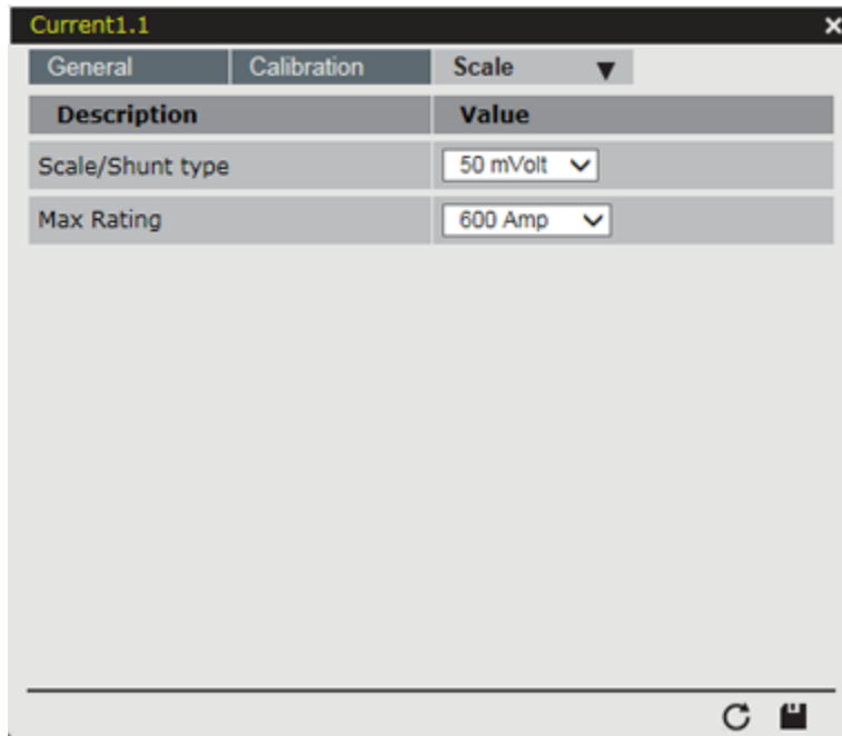
Figure 2.48 - Load Monitor Current Shunt Scale Tab
