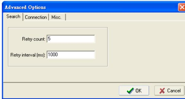
The screenshot shows the 'Advanced Options' dialog box with the 'Search' tab selected. It contains two input fields: 'Retry count' with the value '5' and 'Retry interval (ms)' with the value '1000'. At the bottom right, there are 'OK' and 'Cancel' buttons.
