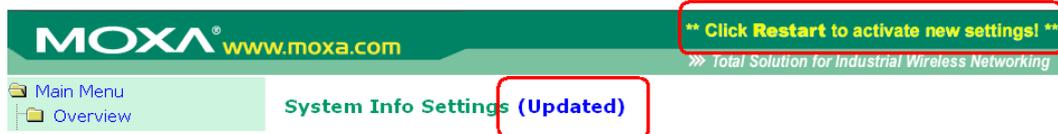
To activate the changes click **Restart** and then **Save and Restart** after you change the settings. About 30 seconds are needed for the AWK-3131 to complete the reboot procedure.
